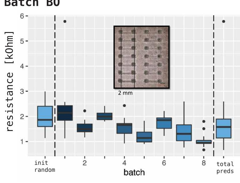
Batch optimization of electrical property of patterned LIG, lower is better. On the left, the distribution of resistance for the initial training data is shown. Each batch has 14 lines (inset); each boxplot represents one batch. On the right, the distribution of measured resistances for all configurations that the MBO explored.
