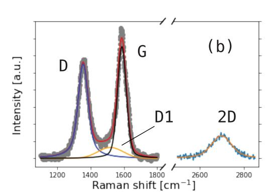
Structural characteristics of LIG (a) before and (b) after patterning of GO. D is attributed to defects. G to in-plane vibrations of sp2 carbon atoms. 2D to stacking order of carbon planes. D1 to amorphous carbon.
