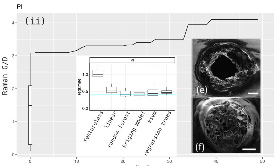
Single-step optimization of the structural quality of LIG on various precursors (i) GO on quartz and (ii) polyimide; higher is better. Boxplot shows distribution of initial training data. Inset: (Left) Comparison of various model performances (right) Scanning electron micrograph of patterned LIG using (a), (e) random and (b),(f) BO parameters
